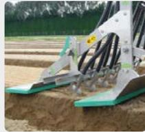
Seed Spider soil openers are unique and designed to form the optimum seed channel with minimal soil disturbance. They form a very fine 'V' shaped slot in the soil for the seed. Soil from one row does not fall onto the neighbouring row, as is the case with most other high density seeders. This ensures even seeding depth across the entire seed bed. The soil openers are also staggered to prevent the build-up of trash
